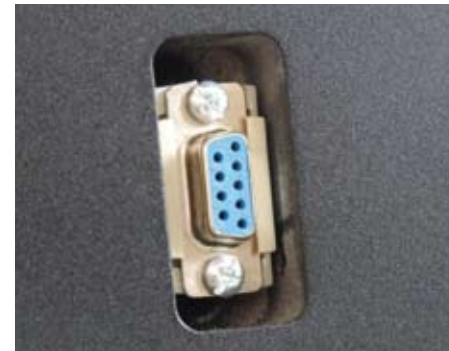
The IR receiver on the top plate relays its signals to the array motors via an RS232 connector.
